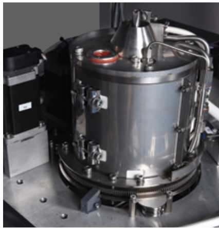
Rotatable non-wettable nozzles avoiding operator interference/ maintenance
